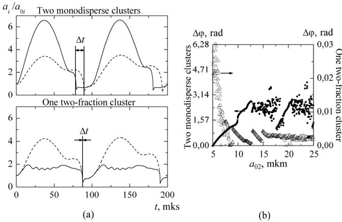
**Figure 4:** Comparison of bubbles oscillations in two monodisperse and one two-fraction clusters at  $\Delta P = 5 \times 10^5 \text{ Pa}$ ,  $\omega = 2\pi \times 20 \text{ kHz}$  and  $N = 10^4$  ( $N_1 = N_2 = N/2$ ):
