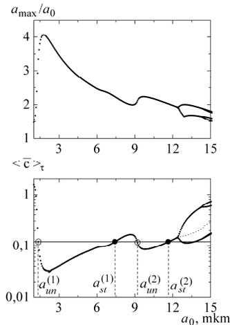
**Figure 7:** Normalized maximum radius (top) and averaged gas concentration near the bubble wall (bottom) vs. initial radius for pressure amplitude  $\Delta P = 1.5 \times 10^5$  Pa.
