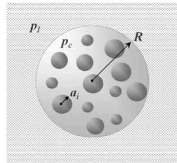
**Figure 1:** Schematic of a polydisperse bubble cluster.
