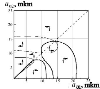
**Figure 8:** The equilibrium curves for bubbles in two-fraction cluster for  $\bar{c}_\infty = 0.12$ .
