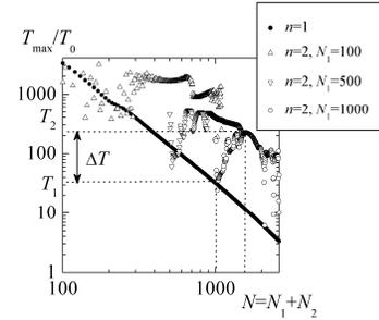
**Figure 5:** Maximum temperature in the bubble of initial radius of  $a_{01} = 5 \text{ mkm}$  vs. total number of bubbles in cluster at  $\Delta P = 5 \times 10^5 \text{ Pa}$ . For the case  $n = 2$ :  $N_1$  is fixed,  $N_2$  is variable,  $a_{02} = 10 \text{ mkm}$ .
