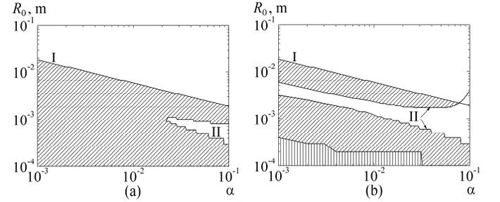
**Figure 2:** Areas of validity of mathematical model shaded by parallel lines for: (a)  $a_0 = 5$  mkm and (b)  $a_0 = 25$  mkm. The area shaded by parallel vertical lines indicates the area where no cluster exist with these parameters. Level curves: I –  $R_0 = \lambda$ ; II –  $\tilde{\sigma}^{1/2} = l$ .
