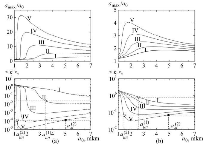
**Figure 6:** Normalized maximum radius (top) and the average concentration of gas near the bubble wall (bottom), depending on the initial radius for different pressure amplitudes:
